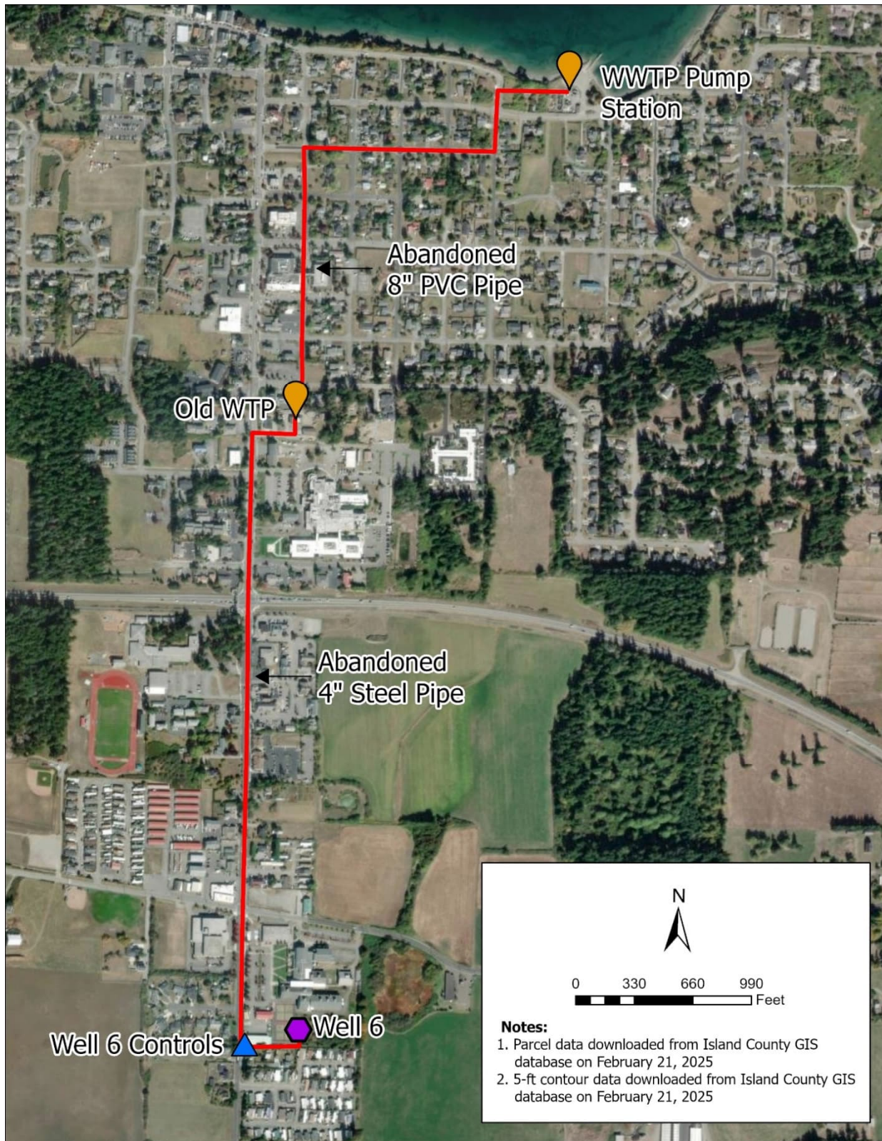
Figure 4-1. Distribution System Existing Conditions
