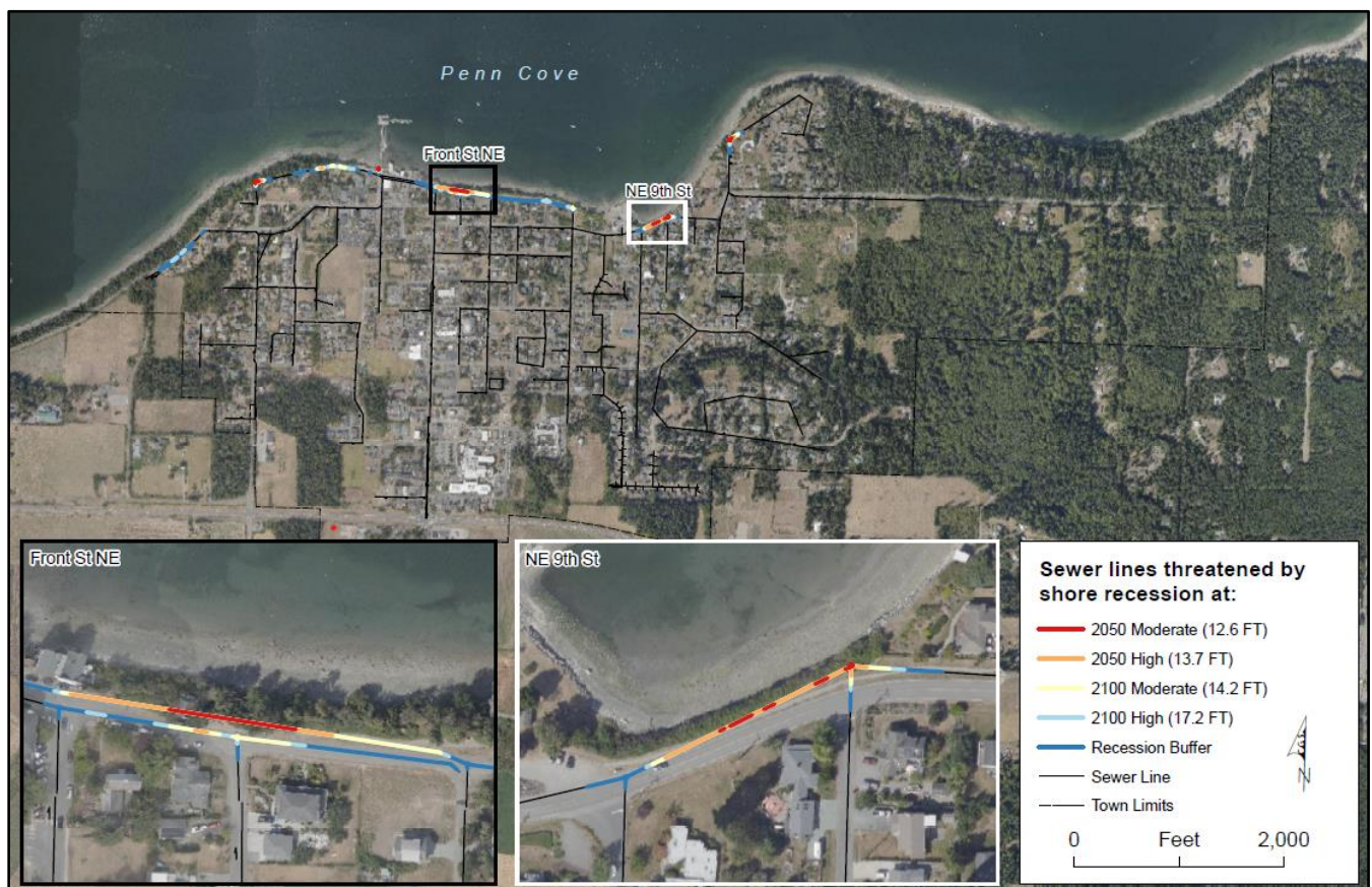
Figure 36. Sewer lines within the Town of Coupeville threatened by shore recession under four sea level rise scenarios (Coastal Geologic Services et al., 2023).
