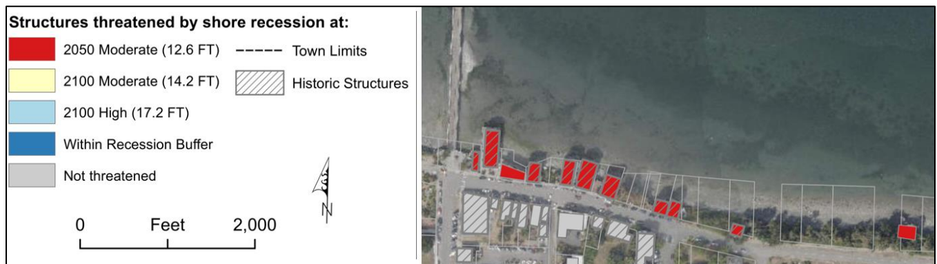
Figure 27. Structures at risk of shore recession from different levels of sea level rise.
