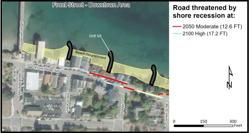
Figure: Conceptual depiction of hybrid shore protection along Front Street and the historic waterfront.
