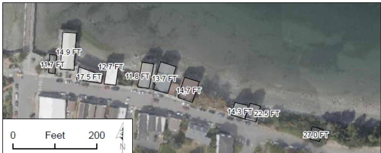
Figure 25. Approximate lowest floor elevations (NAVD88) for the overwater buildings in downtown Coupeville. Note: elevations were not surveyed using high accuracy survey equipment and should be resurveyed for future planning.
