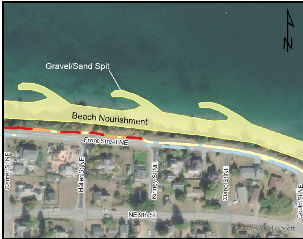
Figure 19. Conceptual depiction of soft shore protection along Front Street – Residential Area.
