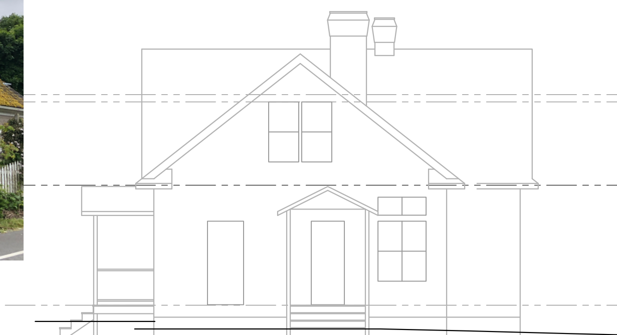
A Existing East Elevation
