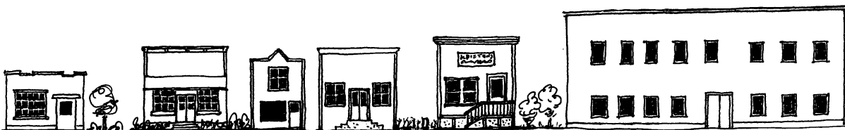
This building is out of scale with adjacent structures, and is not compatible in this setting.
